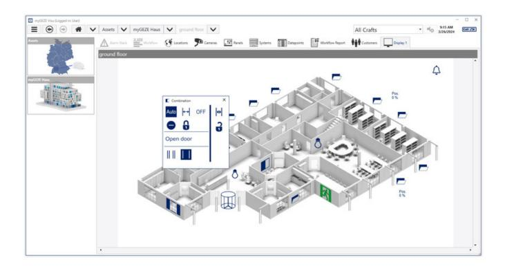
Building management software for visualisation, operation, control and monitoring of connected GEZE product systems
