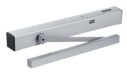
Overhead door closer with guide rail for single leaf doors up to 1400 mm leaf width with electric free swing function and smoke switch control unit transom installation hinge side
