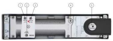
1 = Latching action setting | 2 = Closing speed setting | 3 = Hold-open function setting / closing delay | 4 = Closing force setting | 5 = Frontal gearing pivot
