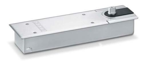
Floor spring for single leaf single and double-action doors of up to 1400 mm leaf width with adjustable closing force EN 3-6 and with hold-open function that can be switched on and off
